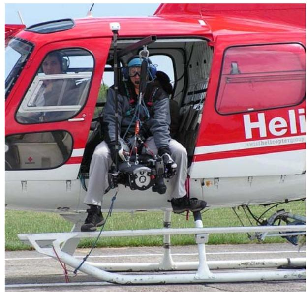
Figure 1: System in nadiral configuration.
