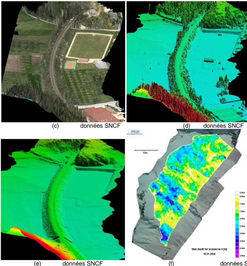
Figure 5: Power lines mapping (a). By flying at 100m above ground, it is possible to detect wires, pylons and obstacles. Steep slopes mapping (Grimsel-Furka road) for 3D road model (b). Orthophoto draped on DSM (c)/DSM (d) / DTM (Laser filtering) of railways (SNCF) (e) / Snow volume measurement of a slab avalanche (vallée de la Sionne, VS) (f).
