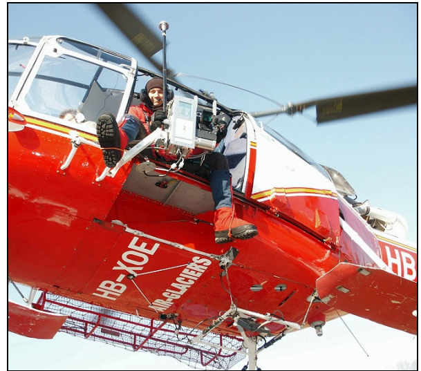
Figure 3: The system in action with Alouette III helicopter. The holder for supporting the system weight during transition flights is located under operator's right leg.
