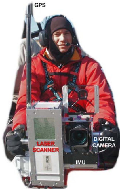
Figure 1: The handheld block composed of all the devices: digital camera, laser scanner, GPS antenna and IMU
